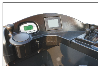
Camera and positioning: Optional positioning system offers easier pallet handling at height through camera system.
